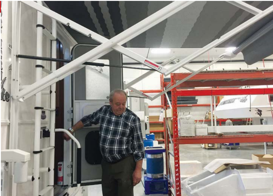
The new production line includes the latest innovations in RV manufacturing. Above, Mac Donkin demonstrating the 7-foot automatic awning, and top right - rear bumper step with patio.
